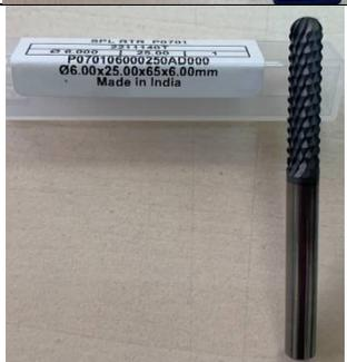
A photograph of a blue end mill with a silver cutting edge. The label above it reads: SPL RTR P0701, 22111887, Ø 6.000, 25.00, 1, P070106000250AD000, Ø6.00x25.00x65x6.00mm, Made in India. |
