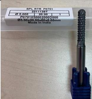
A photograph of a blue end mill with a silver cutting edge. The label above it reads: SPL RTR P0701, 22111887, Ø 5.000, 20.00, 1, P0701050002000D000, Ø5.00x20.00x60x6.00mm, Made in India.  |
