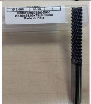
A photograph of a black end mill with a diamond coating. The label on the packaging reads: CONTOUR RTR M P0801, 22111221, Ø 8.000 35.00 1, P0801080003500D000, Ø8.00x35.00x75x8.00mm, Made in India.      |
