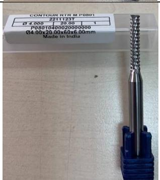
A photograph of a silver-colored end mill without a coating. The label on the packaging reads: CONTOUR RTR M P0801, 22111231, Ø 4.000 20.00 1, P08010400020000000, Ø4.00x20.00x60x6.00mm, Made in India. |
