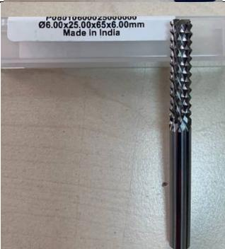
A photograph of a silver-colored end mill without a coating. The label on the packaging reads: CONTOUR RTR M P0801, 22111241, Ø 6.000 25.00 1, P08010600025000000, Ø6.00x25.00x65x6.00mm, Made in India. |
